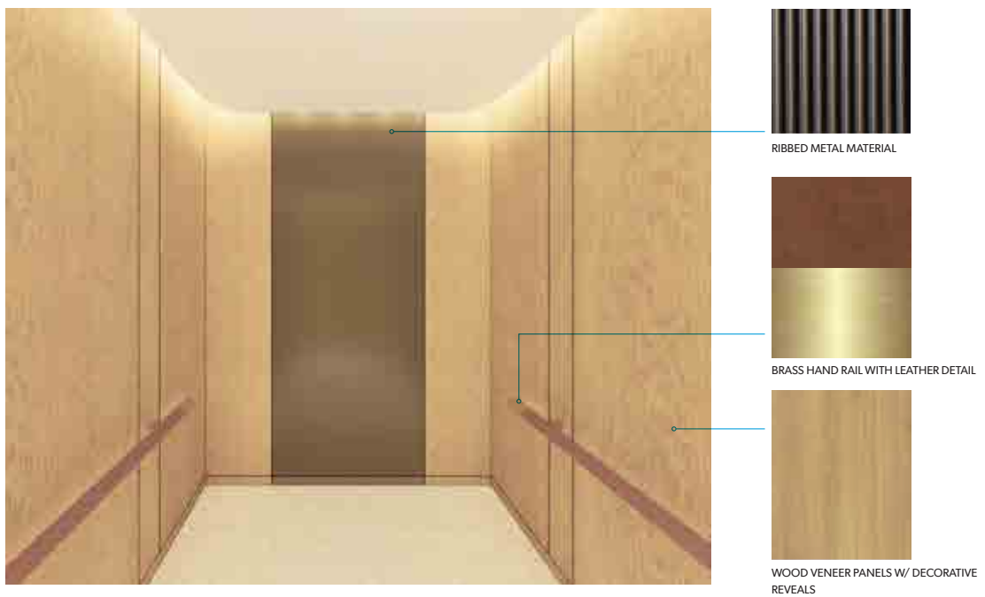
5 | ELEVATION - ELEVATOR CAB WEST 3/8" = 1'-0"
